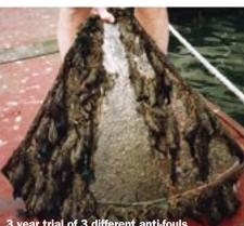
3 year trial of 3 different anti-fouls. Coppercoat is in the centre
